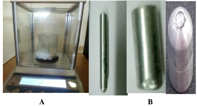
Fig 3.2.1 Density Test A) Experimental Setup B) Sample Specimens
