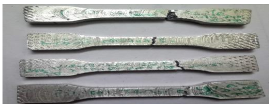
Fig 3.1.1 ASTM: E8/E8M-11 standards Tested Tensile Specimens and setup.
