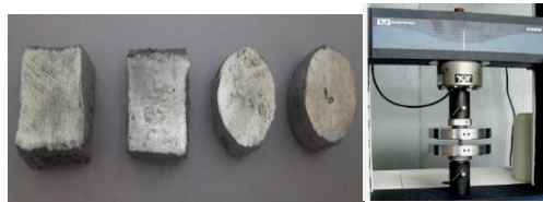
Fig 3.3.2 Compressed Specimens and setup on UTM
