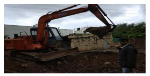
**Hydraulic Excavators-** excavators are also called diggers or shovels. These machines are used for digging trenches and foundations, demolitions, landscaping, and mining projects. Excavators can come in four sizes- mini, small, medium and large.
